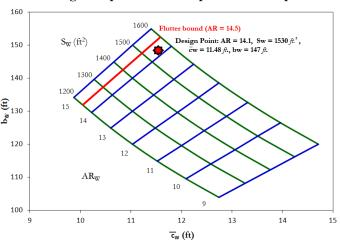
Fig. 58 Parametric study of aspect ratio vs. wing area. The flutter bound for a fully composite wing is shown in red and
