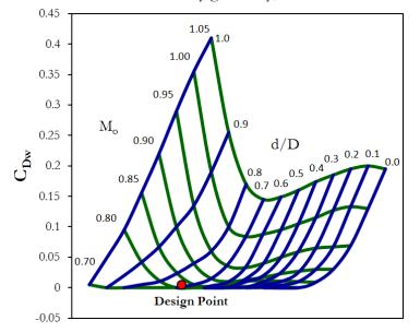
Fig. 12 Forebody Wave Drag Coefficient Vs. Cruise Mach Number (M<sub>o</sub>) and Bluntness Ratio (d/D). The bluntness ratio corresponding to the lowest wave drag coefficient was chosen as the design point.
