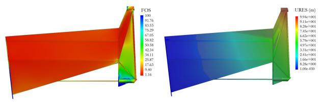
Fig. 35 FEA of aft-mounted engine pylon showing contours of factor of safety (left) and maximum displacement (right)
