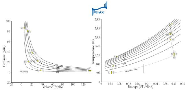
Fig. 27 Basic core cycle shown in PV (left) and TS (right) diagrams.
