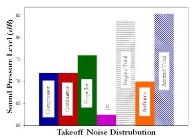
Fig. 70 Maximum sideline noise distribution for Ibis during takeoff. The jet contribution is relatively negligible. The propeller contributes the most to overall aircraft noise.
