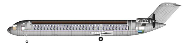
Fig. 50 Inboard profile of Ibis featuring water and waste systems along with piping.
