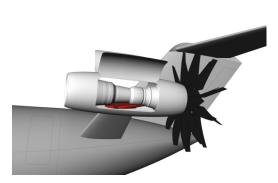
Fig. 39 The engine core accessibility
