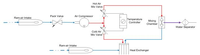
Fig. 42 Air conditioning pack flow diagram. Notice that the recirculation/filtration system is not shown here to be concise.
