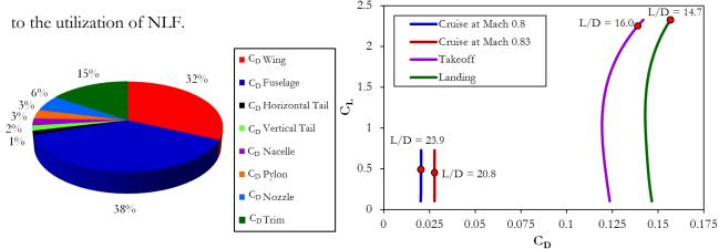
Fig. 23 Drag breakdown at cruise.
