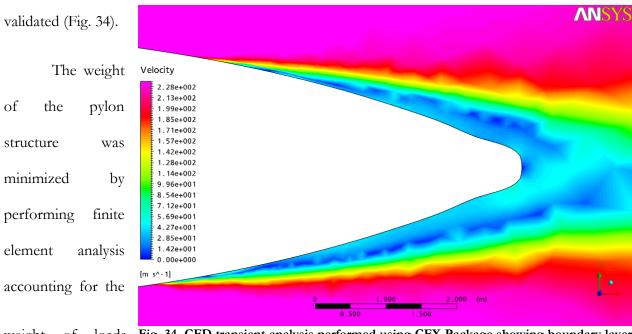
weight of loads Fig. 34 CFD transient analysis performed using CFX Package showing boundary layer thickness around fuselage tailcone at takeoff.
