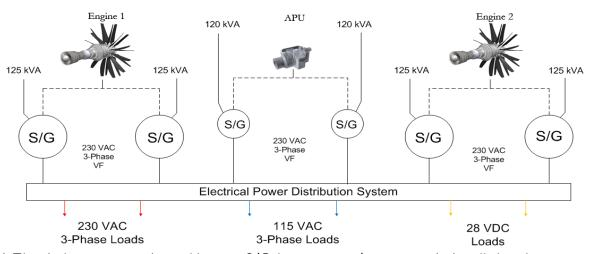
Fig. 41 Electrical power generation architecture. S/G denotes starter/generator units installed on the engines and APU. V/F denotes variable frequency.
