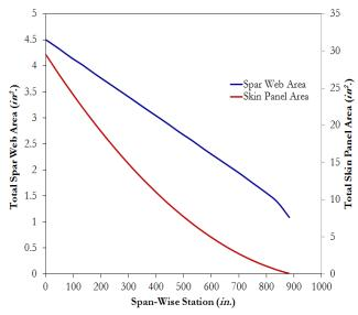
Fig. 57 Spar web & skin panel area vs. span-
