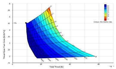
Fig. 38 NOx intensity contours plotted over engine performance map
