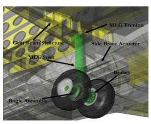
Fig. 45 Main landing gear
