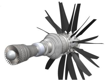
Fig. 5 Open fan engine, pusher configuration
