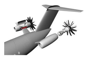
Fig. 40 Engine core detachment
