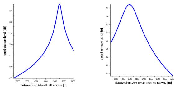
Fig. 69 Flyover noise as measured from 6500 *m.* from the takeoff roll. Maximum sound pressure level is 88 *dB* (left). Approach noise as measured 2,000 *m.* from the 300 *m.* mark. Maximum sound pressure level is 87 *dB* (right).
