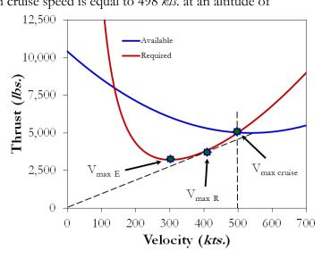
Figure 72. Available and required thrust versus velocity (*cruise*)
