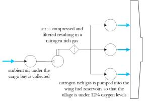
Fig. 48 The architecture of the inert gas generation system providing a nitrogen-rich gas mixture to wing fuel tanks
