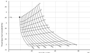
Fig. 31 Propeller map used for engine performance analysis
