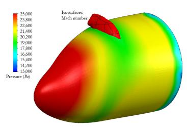
Fig 13 Total pressure contour on the forebody geometry suggests that a favorable pressure gradient is achieved up to the first green area, therefore allowing for possible maintenance of laminar flow. A slight shock is observed on the crown.
