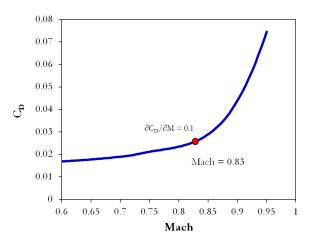
Fig. 25 Result of drag divergence analysis on Ibis indicating a  $M_{DD}$  of 0.83, according to the criteria of  $\partial C_D/\partial M$  of 0.1.
