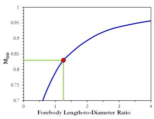
Fig. 11 Drag Divergence Mach Number vs. Forebody L/D
