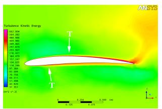
Fig. 14b Turbulence Kinetic Energy for wing root airfoil Fig. 15b Turbulence Kinetic Energy for wing tip airfoil
