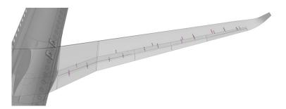
Fig. 43 Location of control surface actuators and flap track fairings
