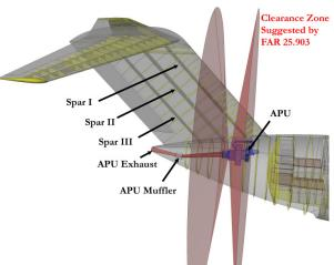
Fig. 49 APU installation showing the FAR §25.903 clearance zone for turbine equipment. In the event of turbine blade loss, there are at least two spars to keep the empennage intact.
