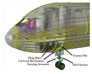
Fig. 44 Nose landing gear
