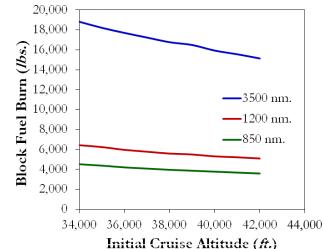
Figure 73. Block fuel burn vs. initial cruise altitude for ranges of 3,500 nm., 1,200 nm., and 850 nm.
