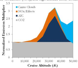
Fig. 64 Environmental multiplier vs. altitude
