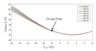
Figure 17 indicates that as the Fig. 17 Variation in cruise L/D as a result of changes in the sweep of the wing, performed using the dynamic spreadsheet. The design point is defined by susceptibility to flutter and divergence.
